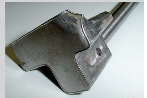
Deposit welding on worn waterproof edges (Photo: L&A Lasertechnik, Radebeul)
