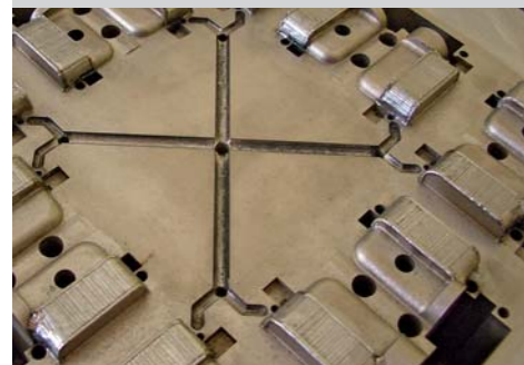
Multi-layer welding to re-shape an 8-cavity mould (Photo: Jutz Lasertechnik GmbH, Wien)
