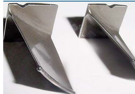
Repair of damaged contours on turbine flaps (Photo: L&A Lasertechnik, Radebeul)
