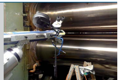
Repair welding on roller (Photo: tcms, Gummersbach)
