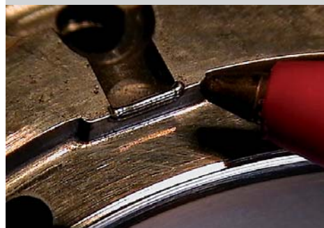
Copper-Berillium-welding (Photo: USMWA of NC, USA)
