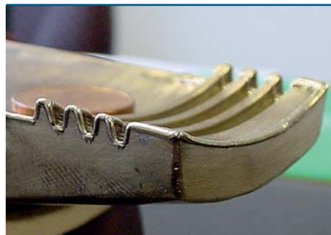
Restoration of worn waterproof edges of a mould element of Ampco-Bronze (Photo: L&A Lasertechnik, Radebeul)
