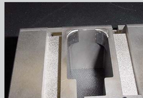
Changing the radius on the matrix of a punching tool of 1.2379 (Photo: L&A Lasertechnik, Radebeul)
